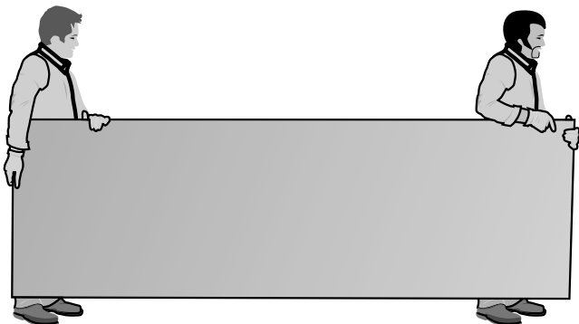
Figure 5 – Final slab lifting phase to vertical position when the slab is in vertical position, lift it from the upper edge and move, taking care to keep it straight at all times (see fig. 6).
