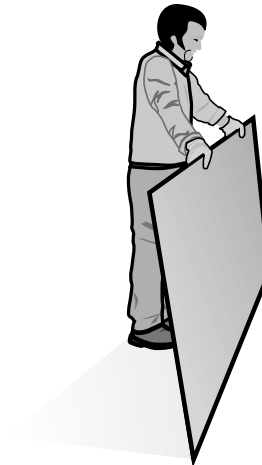
Figure 7 – Initial slab horizontal positioning phase. Then slowly lower the slab onto the flat surface (see figs. 8 and 9).
